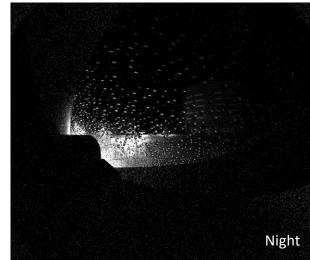
Headlamp outer lens with 3M hydrophobic film
